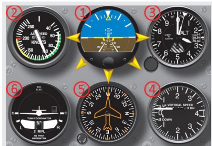
Figure 1: Steam gauges (Morris, 2017).
