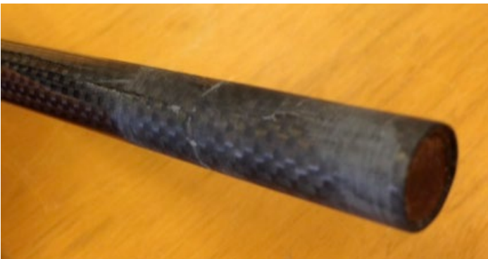
FIG. 3 WOOD DOWEL INSERTED AND BONDED WITHIN DAMAGED CARBON FIBER TUBE (LEASURE)
