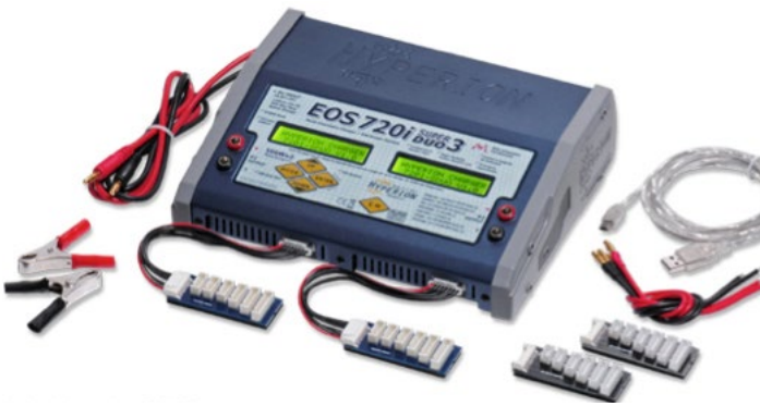
FIG. 4 LITHIUM POLYMER CHARGER WITH BALANCING PORT CAPABILITY, (HYPERION MEDIA)
