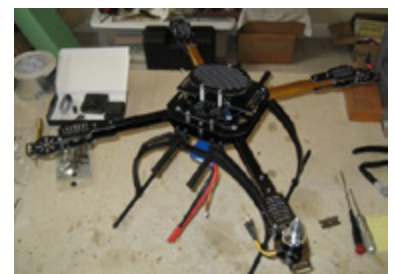
The structural frame is completed with electronics and power system installation pending.
