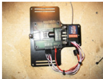
Flight stabilization board (avionics) with manual flight control receiver mounting to airframe hub.
