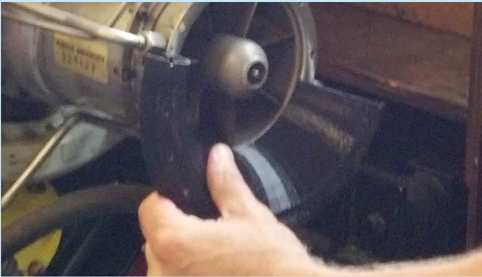
Figure 6. 3D printed bellmouth inlet installation.
