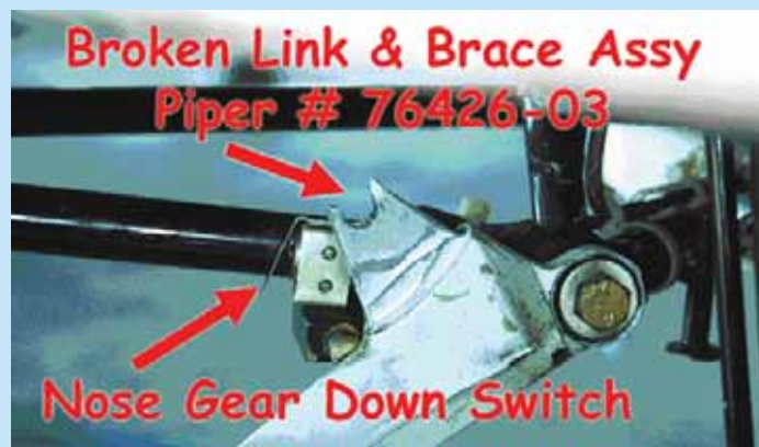
Figure 2: Broken Connection Point for Hydraulically Actuated Down lock Link
