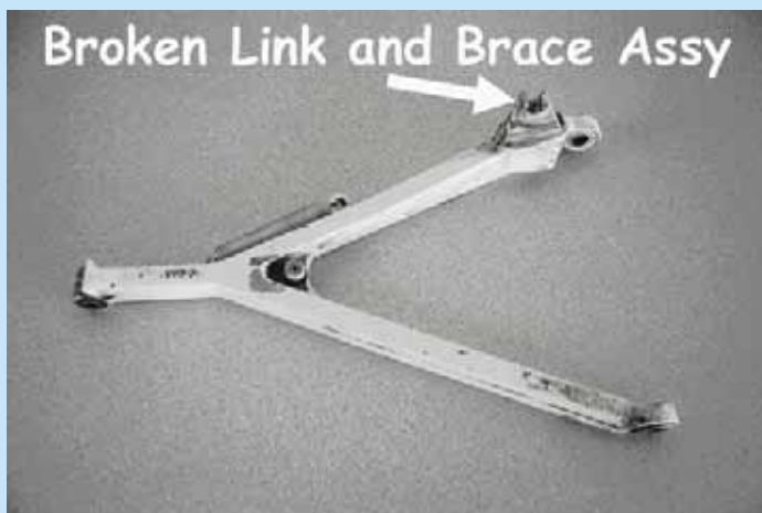
Figure 5: Broken Link Assembly
