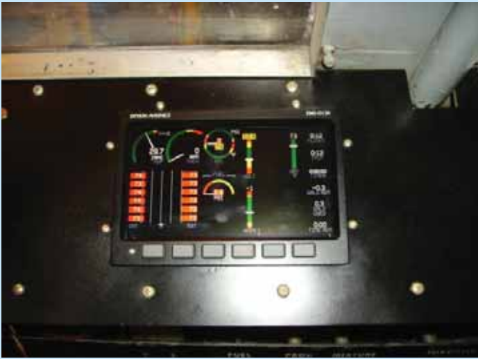
Figures 6 and 7. Depiction of Dynon EMS-D120 display with engine off and engine running (Hannon and Harrison, 2009)
