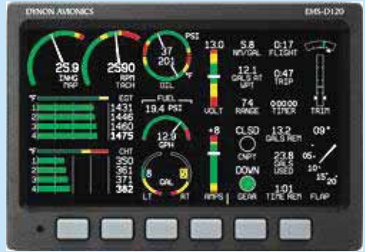
Figures 6 and 7. Depiction of Dynon EMS-D120 display with engine off and engine running (Hannon and Harrison, 2009)
