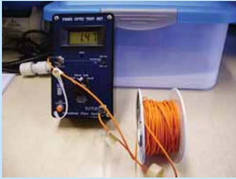
Figure 3. Test Set Up for Glass Core F.O. Cable
