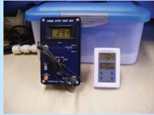
Figure 4. Transmissivity Control and Temperature Humidity Display
