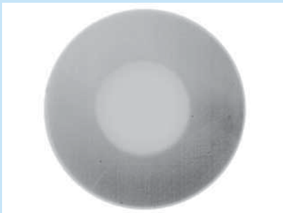
Figure 1. Photomicrograph of Acceptable Polished Glass Core End Face
