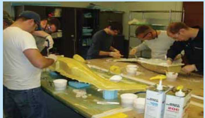
Figure 5. Left, laying up Kevlar on second side of plug. Right, laying up fuselage in new mold.
