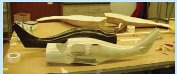
Figure 6. Plug, 2 molds, and first article skins trimmed ready to bond
