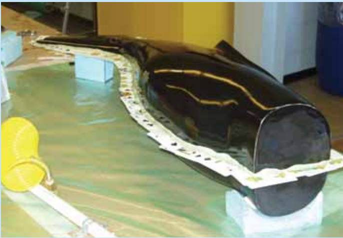
Figure 3. Plug with playing card ledge ready for Layups
