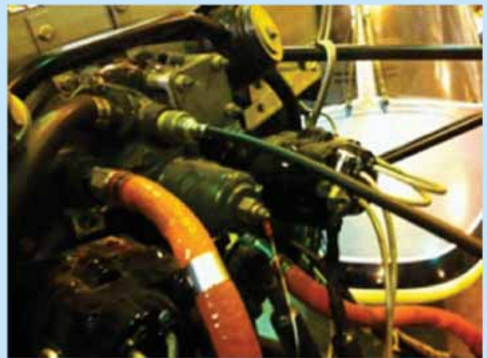
Figure 2. Oil cooler lines to engine
