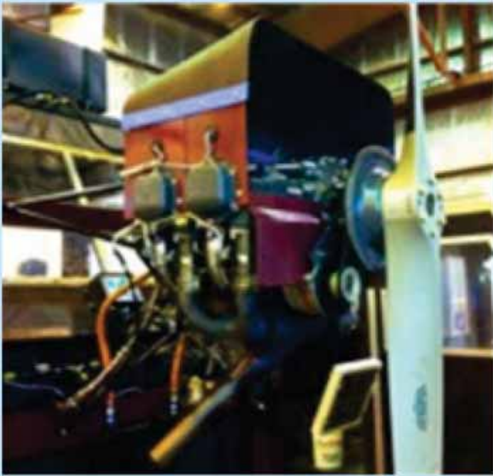
Figure 12. Temporarily Mounted Cowling
