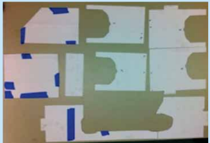
Figure 4. Prototype Cardstock Cylinder Baffling
