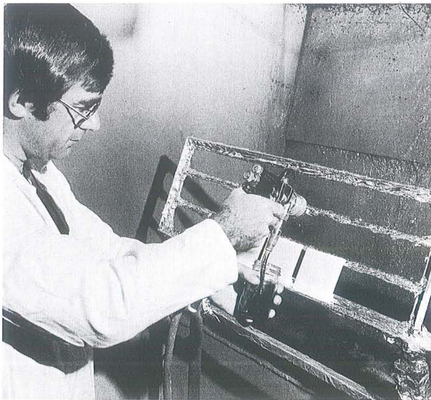
A primer based on CP-153-2 is shown here being applied to the surface of clean, untreated high density polyethylene panels. The tests were conducted in the Technical Service Laboratory of Eastman Chemical Products, Inc.
