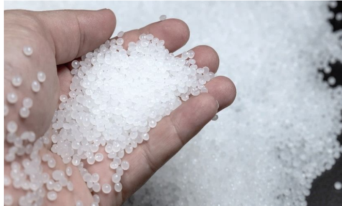
Compounding of PCR granules with new antioxidants and UV protection
