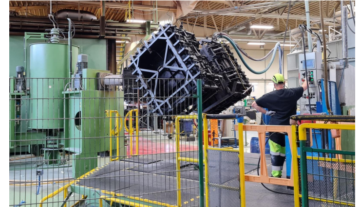
Rotomoulding new Sæplast tubs with PCR content
