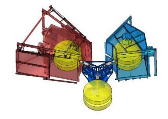
14 min Heat / Cool / Demold66 arms per 24 hours2 operator demolding stations
