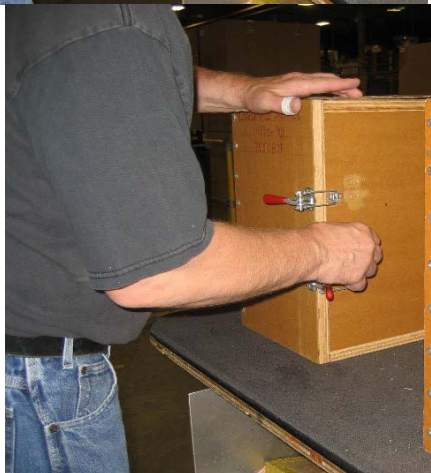
5.2.3 Place the molding into the cooling fixture #7550879 with the front facing outwards then place the front cooling fixture #7550729 into place in the molding. Close and latch the fixture.
