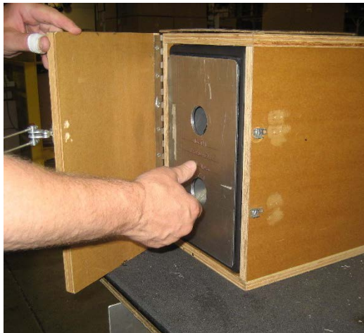
5.2.2 Place the back cooling fixture #7550729 into the back of the molding and tape in place.
