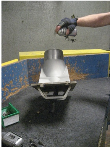
5.1.10 Spray the front cover with Stoner and install it back onto the mold.
