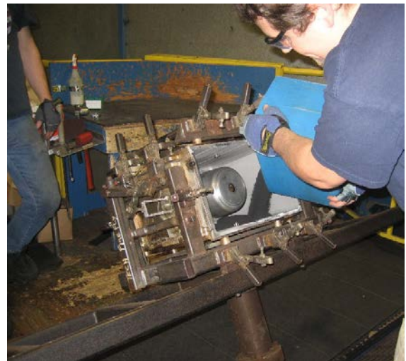
5.1.12 Pour the charge into the mold and distribute evenly.
