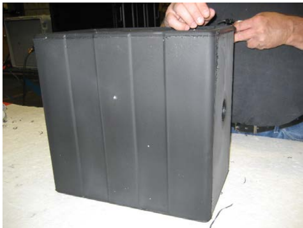
5.2.1 Trim the parting lines on the warm molding.
