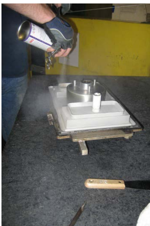
5.1.13 Spray the back cover with Stoner and install it back onto the mold.
