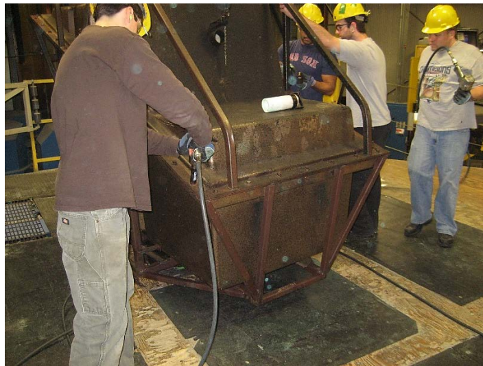
5.1.4 Place the cover onto the can and start bolts by hand and then tighten each bolt starting from the bottom of the cover and moving upwards.
