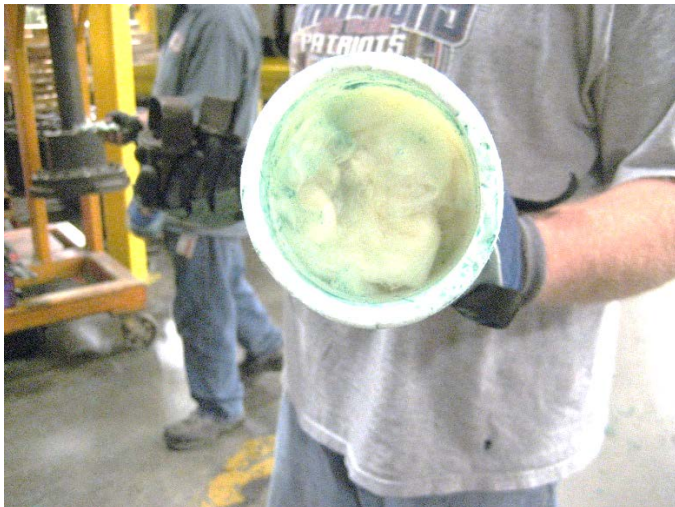
5.1.5 Pack vent tube and install the vent with the hook and utility wire.
