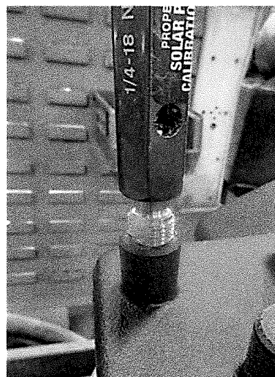
Thread Check with 40542 Thread Gauge
