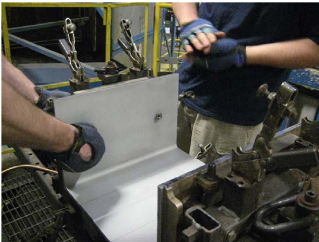
5.1.9 Install all of the T-nuts in the mold according to the print.
