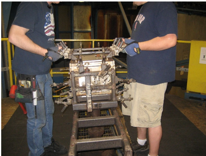
5.1.11 Install the top section back onto the mold.
