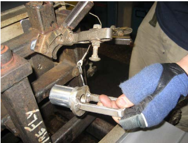
5.1.7 Spray the plug with Stoner and insert it back into the side of the mold.
