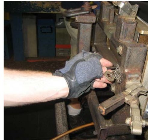
5.1.8 Replace the T handle back into the side of the mold.
