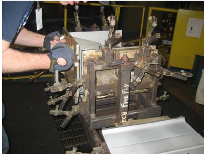
5.1.10 Spray the front cover with Stoner and install it back onto the mold.
