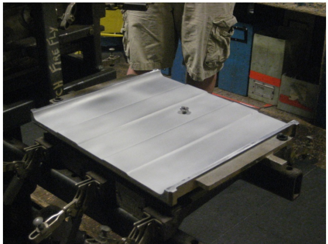
5.1.8 Replace the T handle back into the side of the mold.
