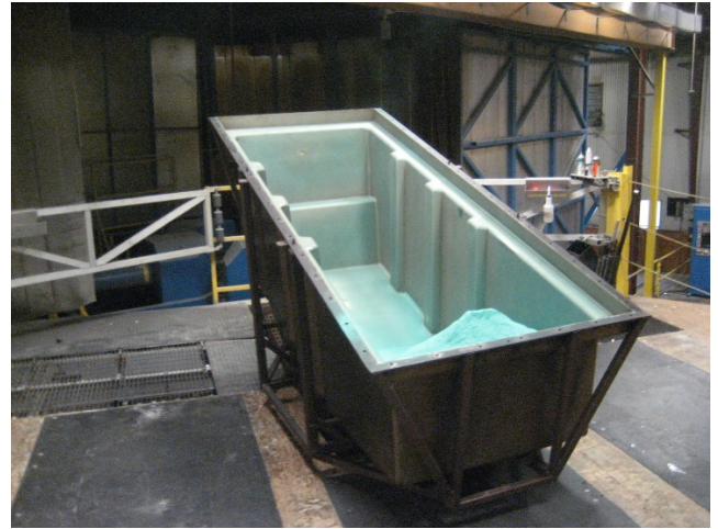
5.1.3 Wipe the parting line with 420 and then load required powder.
