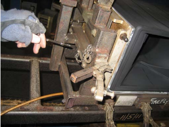
5.1.5 Remove the T handle from the side of the mold.
