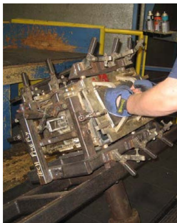
5.1.13 Spray the back cover with Stoner and install it back onto the mold.
