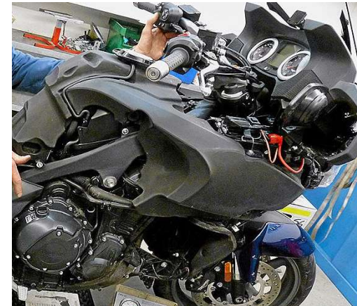
Fuel Tank, XPE (rotational molded)
