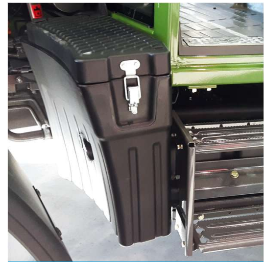
Diesel Tank with storage compartment, PE (rotational molded)
