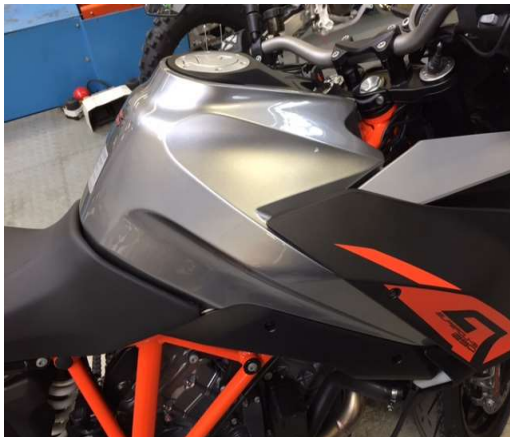
Fuel Tank, PA6 painted (rotational molded)
