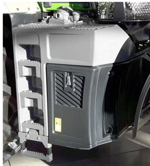
Hydraulic Oil Tank, PA6 painted (rotational molded)
