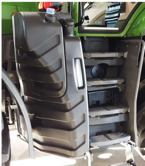
Urea and Diesel Tank, PE (rotational molded)
