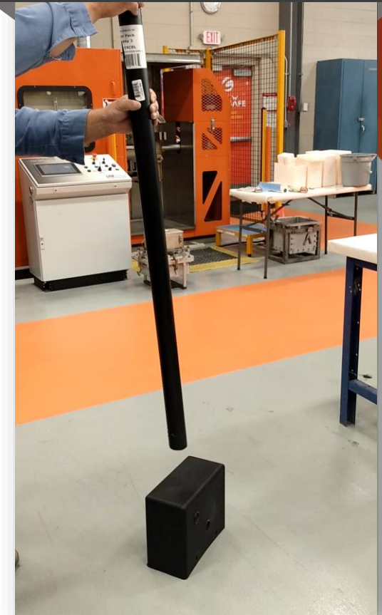
ANSI Tank Impact Test Simulation
