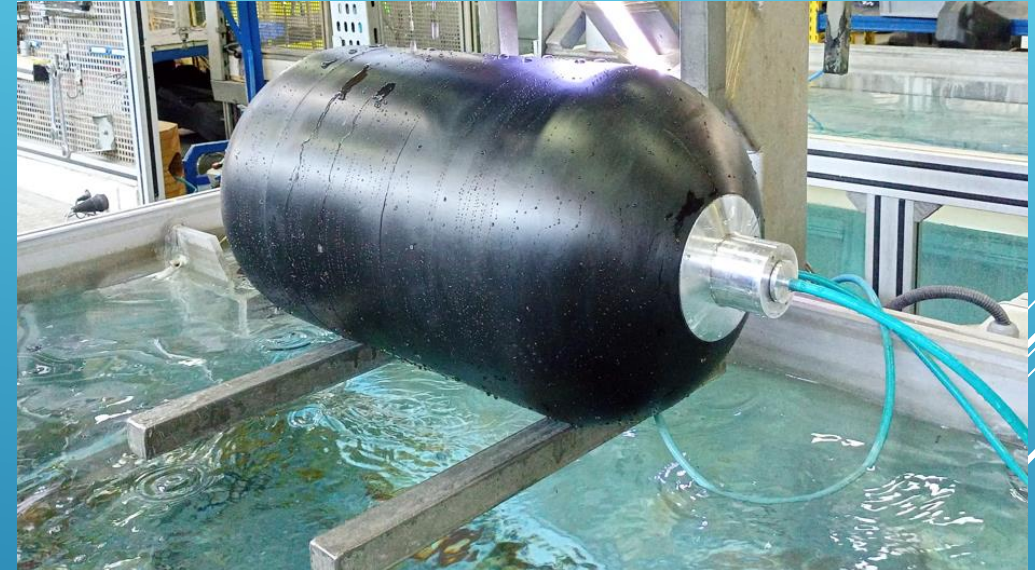
Air Leakage testing of rotomolded liner
