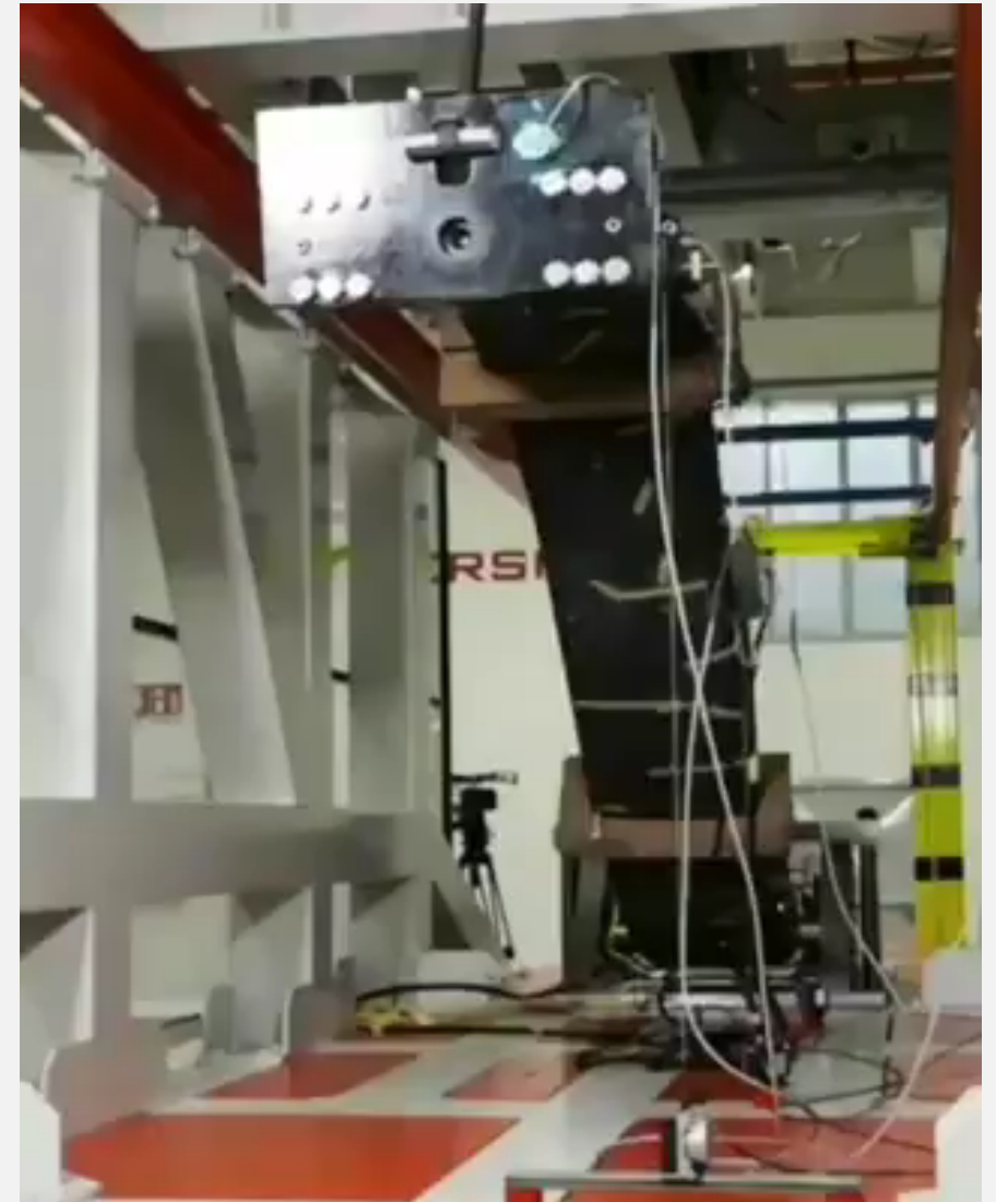
28 ton stress load test on carbon fiber foils
