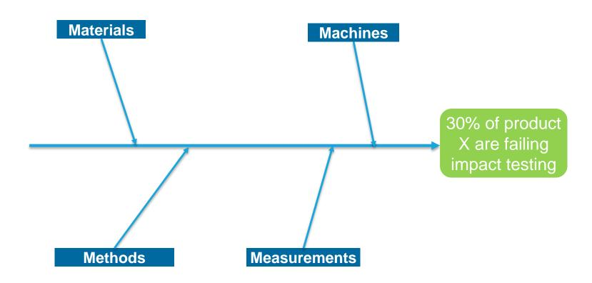
**Example: Poor impact strength cause-effect diagram** Peel back the layer by asking What and Why?
