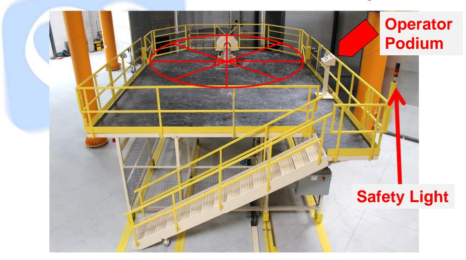
Platform allows access to spider for mold servicing
