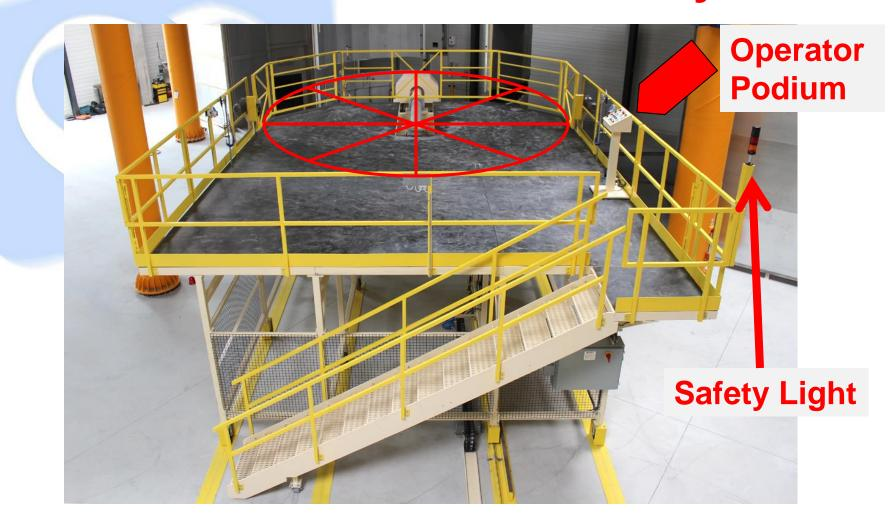
Platform allows access to spider for mold servicing
