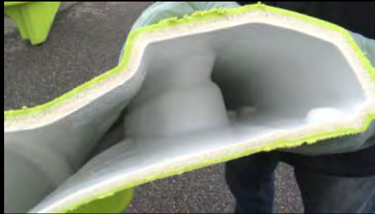
Triple Layer Foam Cross-Section
