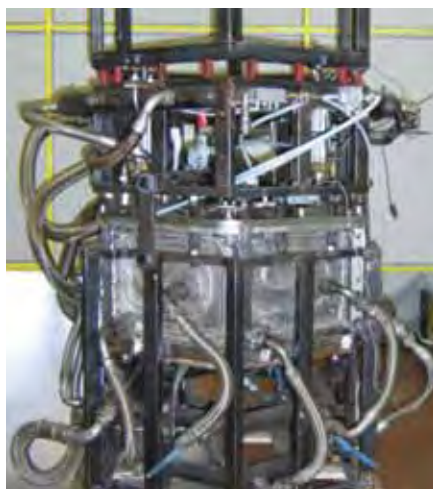
Figure 1: Mould (on left) with pipework to distribute heating and cooling fluid, and moulded part (on right).
