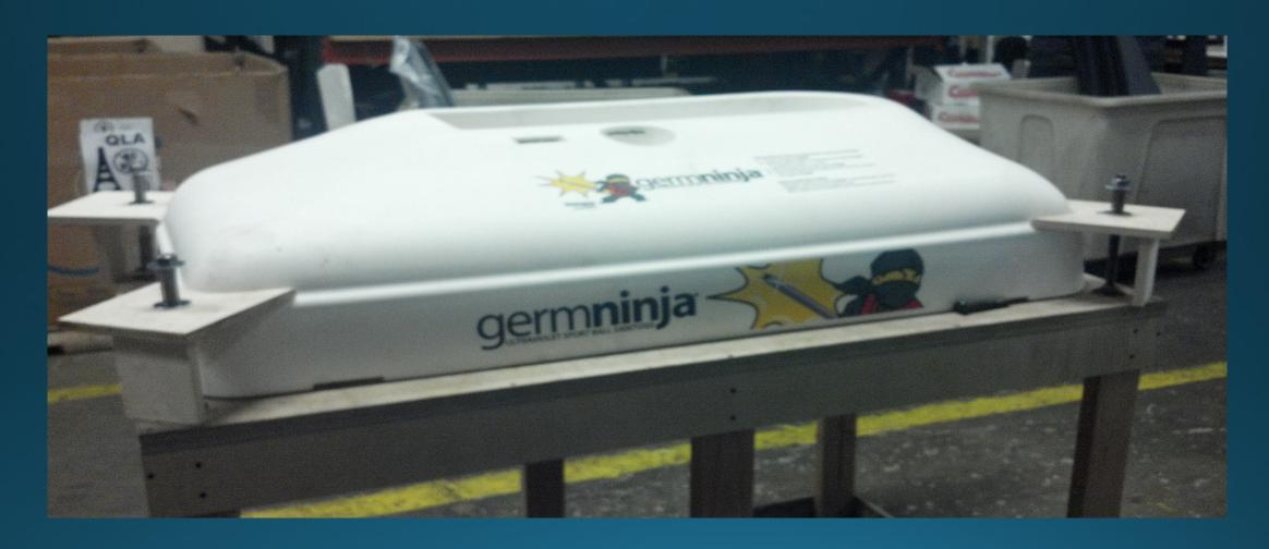
• Spring-loaded clamping system pushes down unit onto flat surface as part cools.
