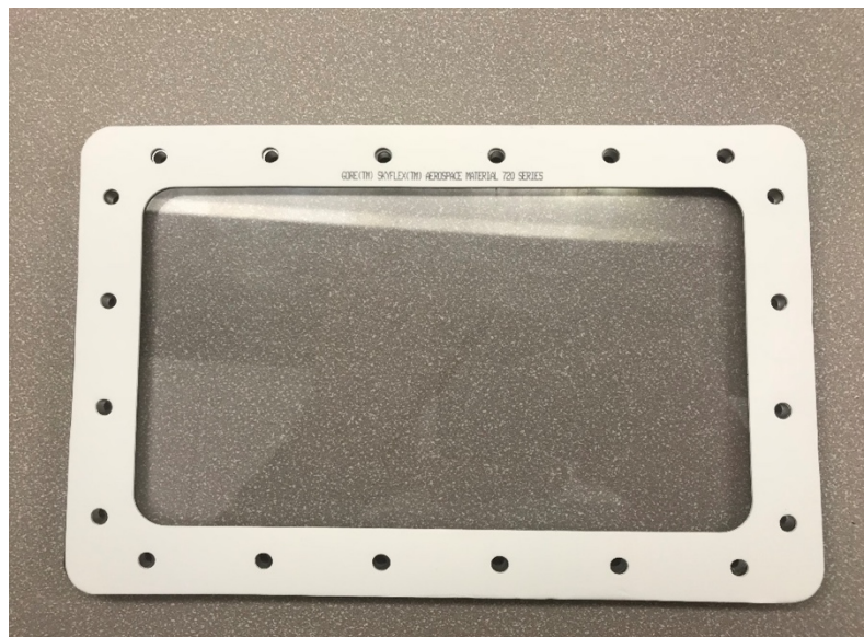
Figure 1 - Shows Gasket installed on Lexan Access panel
