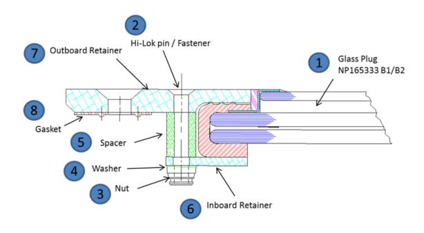
Figure 1 – Window Glass Plug/Retainer Diagram
