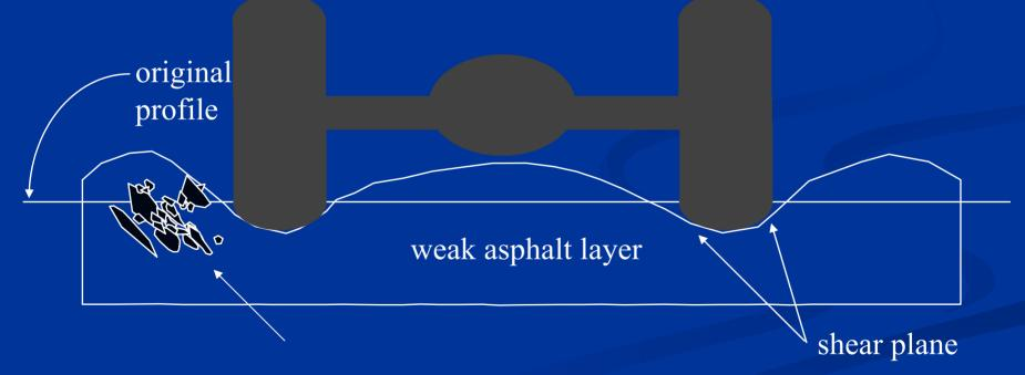
Movement and rotation of aggregate creates very high strain in the binder.
