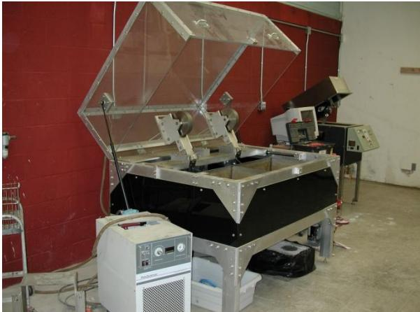
**Hamburg Wheel-tracking Test Results (typ):**
