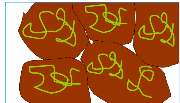
Emulsion of polymer modified asphalt
