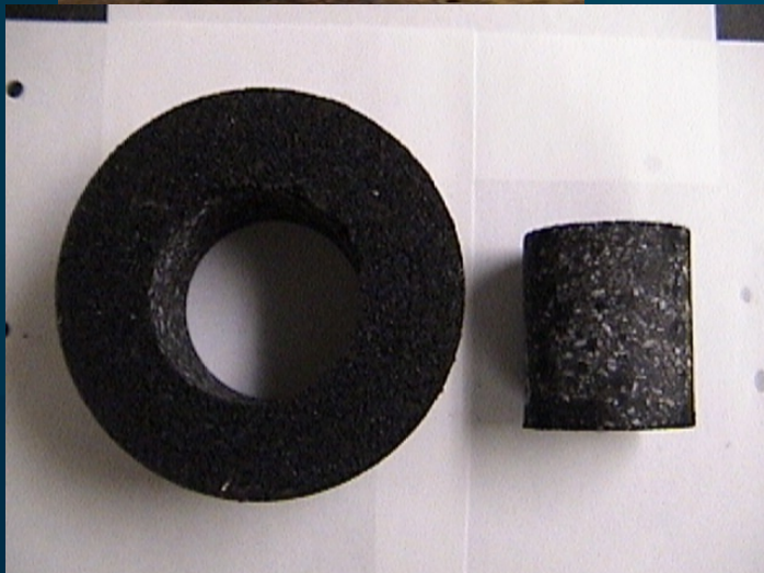
Samples cored from 6-inch diameter gyratory sample
