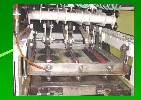
AASHTO TP 63 100 lb wheel load; 100 psi hose pressure Tested at 64°C for 8,000 loading cycles
