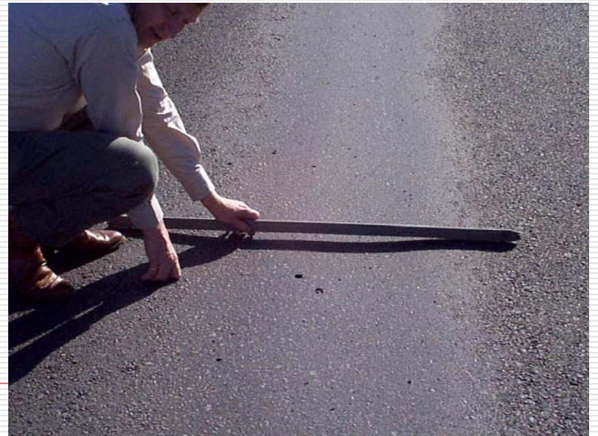
PG 67-22 unmod. 15mm rutting
