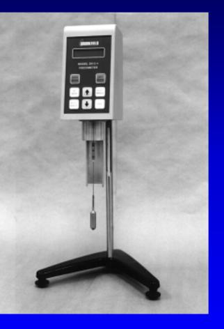
Rotational Viscometer (Brookfield) Viscosity at 135°C and 165°C ➤ Viscosity @ 135°C < 3.0 Pa·s</p> Equi-viscous Lab Mixing and **Compaction Temps** Does not work for PMA - use suppliers' recommendations Not for field temperatures
