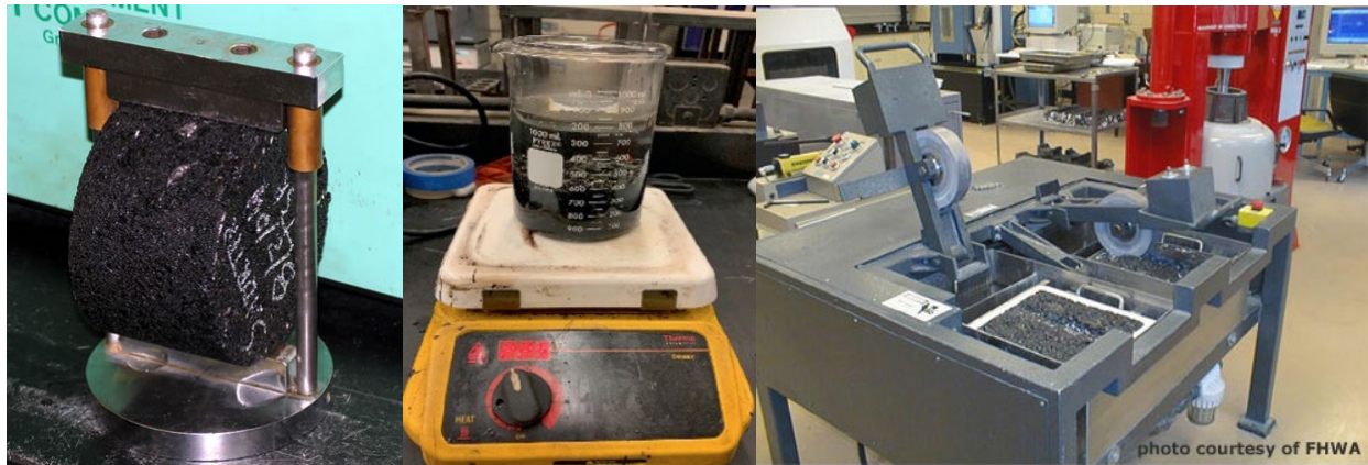
Figure 5. Tests typically used for vetting ASAs by agencies: (left) tensile strength ratio (TSR) test (Pavement Interactive), (center) boil test (Yadav et. al (2022)), and (right) Hamburg wheel tracking (HWT) test (Pavement Interactive)
