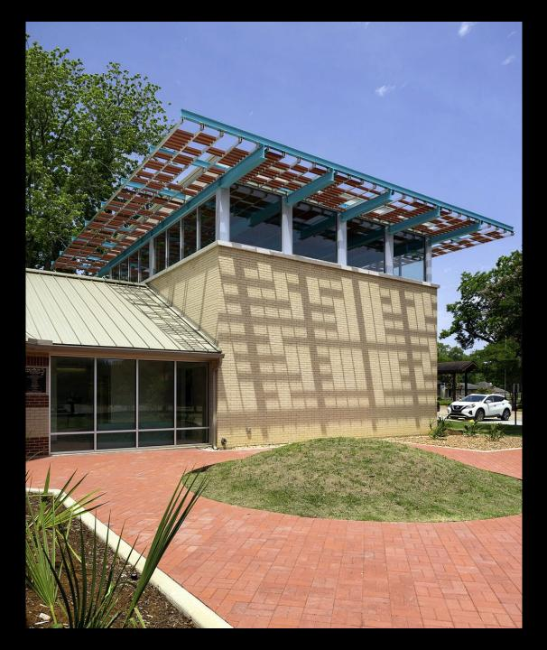
A ceremonial mound anchors the center of the brick-paved plaza, positioned along the approach between the two wings of the building. The brick pavers are laid in a basketweave pattern at a 45-degree angle to the wings in order to align with the lobby's diagonal orientation in plan. The woven brickwork nods to traditional Native craft while marking the transition from landscape to civic space.
