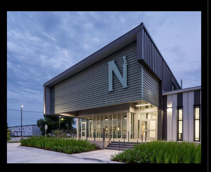
The community façade entry features outdoor café dining under a cantilever roof form. The building is elevated to meet flood elevation requirements. The college logo is prominently displayed on a corrugated perforated metal scrim, offering solar and rain protection while allowing diffused natural light into the café. The metal roof extends down parts of the façade. The landscaping incorporates indigenous plants native to the campus environment.
