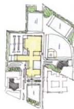
SCHEME 1.0 A two-story scheme with a large footprint. Centralized entry fronting a half-size lawn, which may compromise band practice. A generally north-south arrangement of layered elements forming multiple courtyards. Optimum field orientations.
