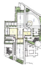
SCHEME 4.0 Gracious courtyard scheme; excessive perimeter. Immediate access to front lawn from school; compromised traffic patterns. Building footprint completely avoids existing building footprint. Compromised solar orientation of some upper-floor classrooms.
