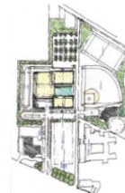
SCHEME 2.0 A more compact three-story scheme (as are all others that follow). Central courtyard has views to ball field. Parking at back of site with optional connection to Patterson Dr.
