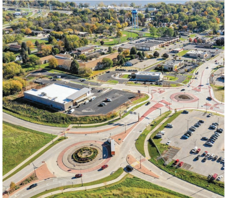
The two roundabouts flow into each other which provides a continuous stream of traffic and reduces the risk of serious accidents.
