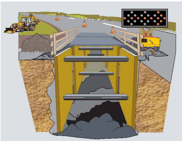
Trenches more than 4' deep meet OSHA's definition of a confined space.
