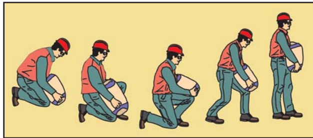
Fig. SS-4B. Use proper lifting technique. Lift with your legs not your back.
