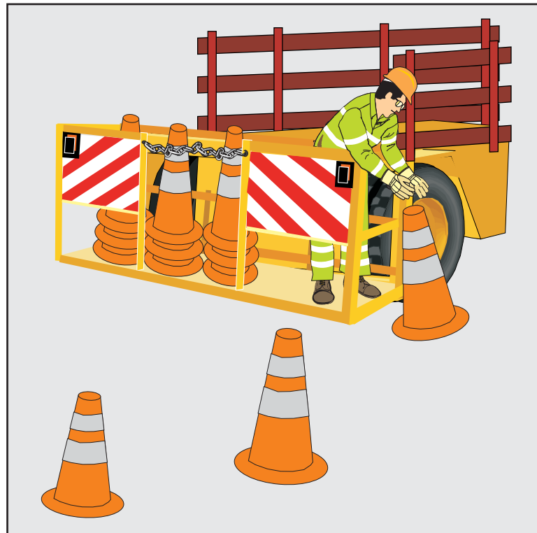
Fig. RB-5. Use seat, seatbelt, fall restraint, or guardrail and a handhold when guardrail must be removed.
