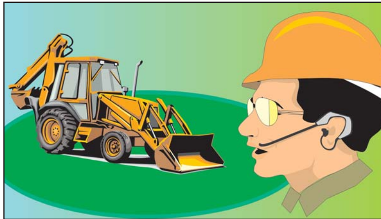
Fig. RB-4. Communicate with the driver or operator and make sure the driver or operator acknowledges you
