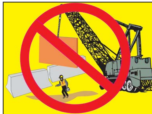
Fig. SC-1B. Keep workers from beneath loads.
