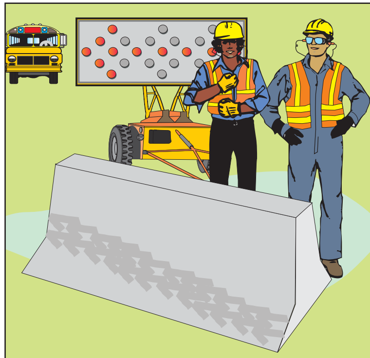
Fig. RB-1. Stay behind protective barriers where possible to avoid death or injury from run over, back over, or roll over of equipment.
