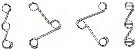
Figure 19: Lock-wiring of bolts
