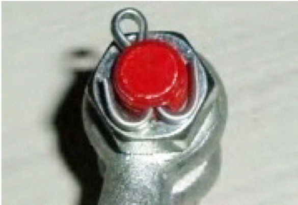
Figure 21: Cotter pin in a shackle bolt
