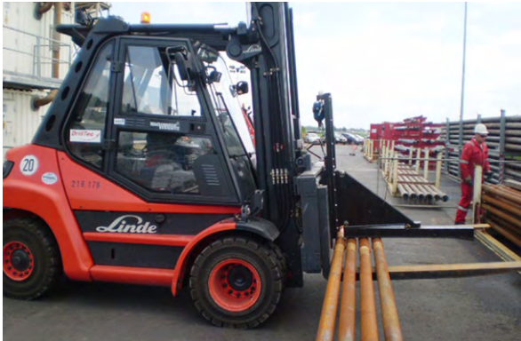
Figure 2: Forklift truck handling tubulars with a clamp
