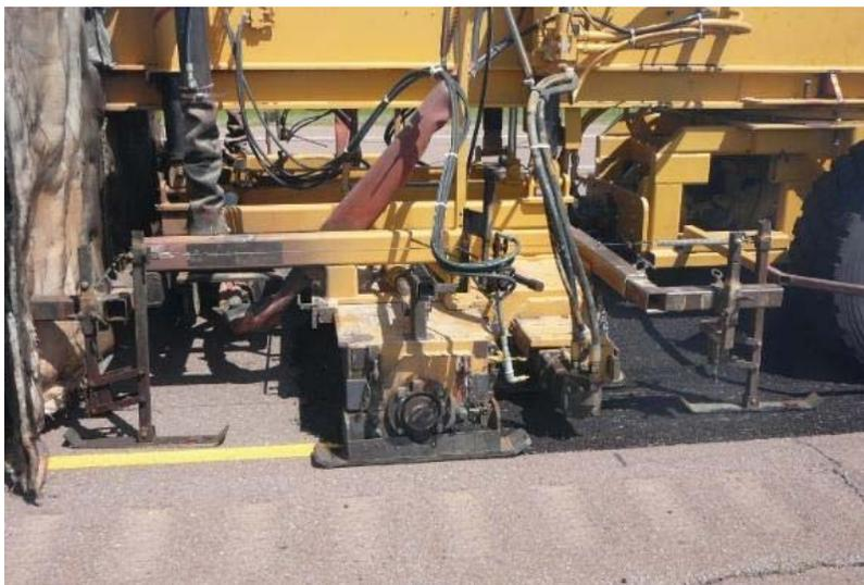
**Figure 13. Low Energy Milling Heads (photo courtesy ARRA)**
