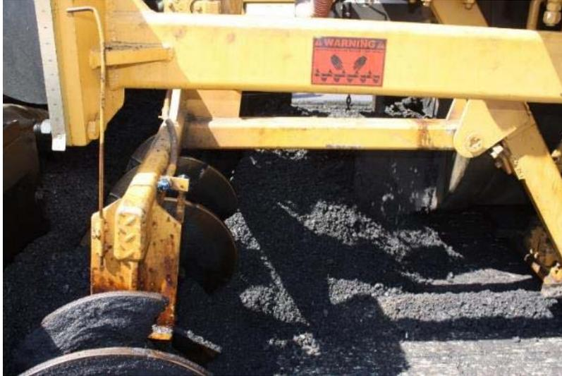
**Figure 14. Auger System (photo courtesy of ARRA)**
