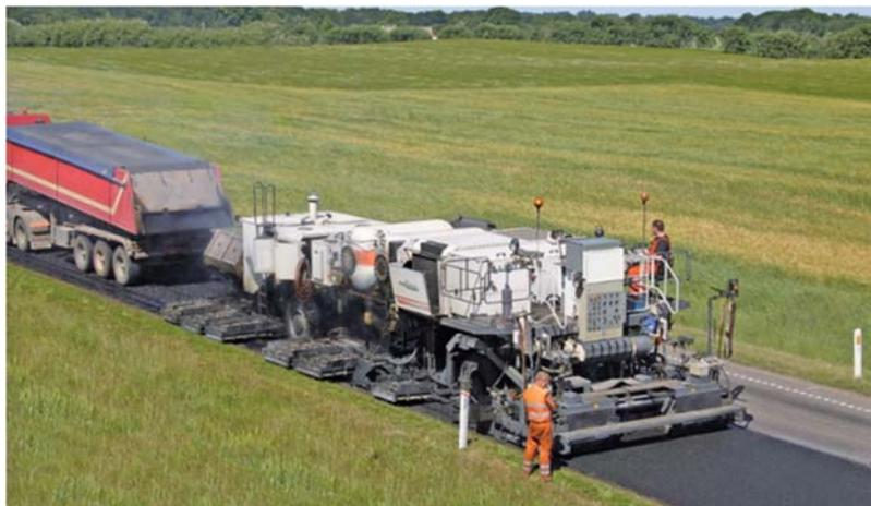
**Figure 17. Remixing Train (photo courtesy of ARRA)**
