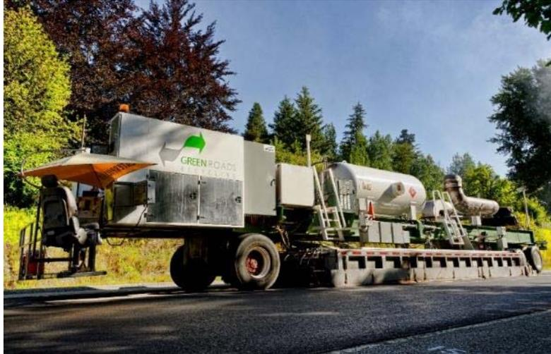
**Figure 11. Typical Preheating Unit (photo courtesy of ARRA)**
