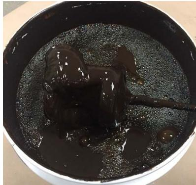
**Figure K.4. Emulsion Sediment in Good Condition**
