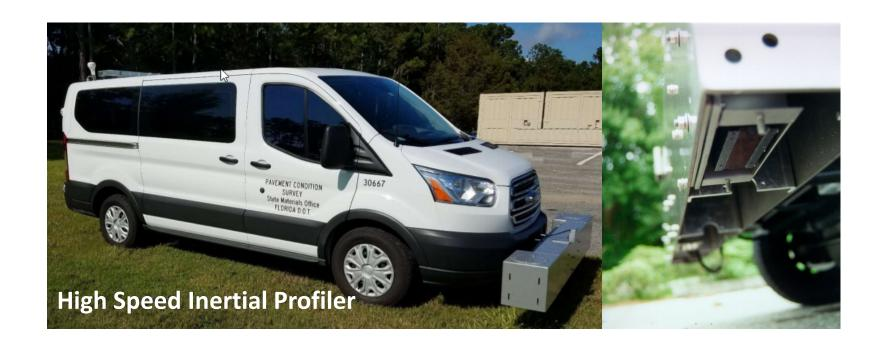
Bumper mounted laser sensors on each wheel-path measure distance to the ground to determine the longitudinal profile.
