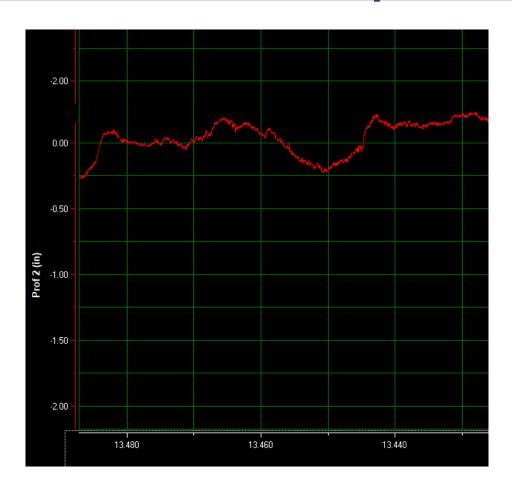
**Smooth pavement**: smaller, flatter, low-amplitude waveforms
