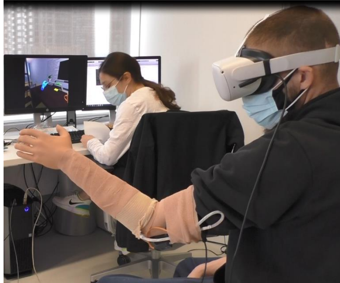
Figure 1. The experimental setup as shown while a subject is immersed in the VR world and completing one calibration of TBC, visible on the left computer screen, on Day 2 of the study.
