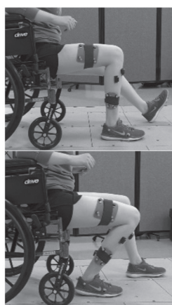
Figure 2. Ankle stiffness testing procedure.
