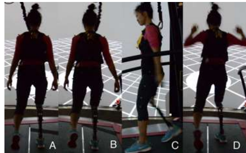
Figure 1. Amputee subject on the CAREN system, which can simulate perturbation and walking scenarios by A) Rolling to the left, B) Rolling to the right, C) Pitching down (or up), and D) Creating a foot slip scenario by suddenly stopping one side of the treadmill. These are just 4 examples of the many scenarios it can simulate. Coupled with a visual environment CAREN can safely record video and biomechanical analysis of an intervention's effectiveness in a multitude of environments.
