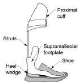
Figure 1: The IDEO-heel wedge-shoe system. Compression of the heel wedge under the IDEO simulates plantarflexion during loading response and allows smooth forward progression.
