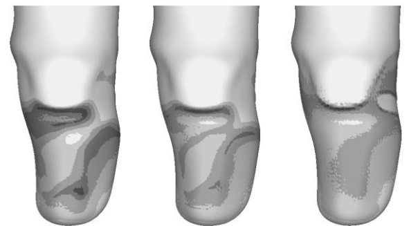
Figure 2: Frictional shear stresses for hard-slick (left), soft-slick (middle), and soft-sticky (right) liners
