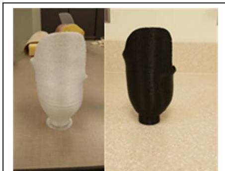
Figure 1. Transtibial Sockets made using the Rostock Max V2 printer. The left image was made using the PC-Plus filament and the socket in the right image was made using ABS.
