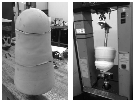
Figure 1: Left: Residual limb model with the divided liner. Right: Adaption of ISO 10328 Configuration 1.
